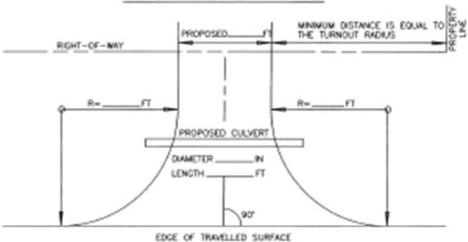
NOTE: LOCATE THE PROPOSED CENTERLINE OF THE ENTRANCE WITH A STAKE, LATHE, OR PAINT SO THE ACTUAL LOCATION OF THE ENTRANCE CAN BE ASSESSED FOR PERMIT APPROVAL.
