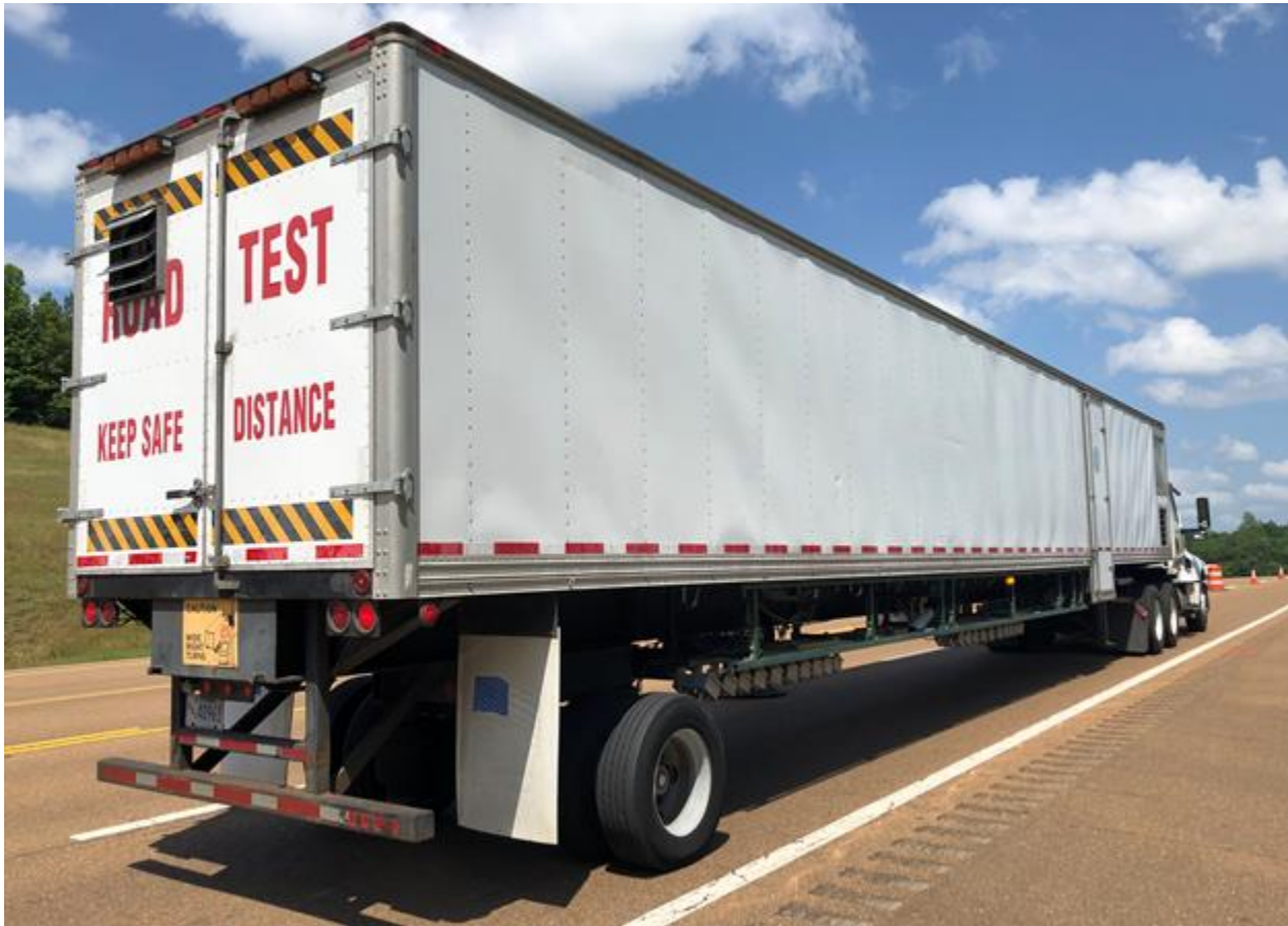
Figure 3. ARA performs structural testing with the RWD.
