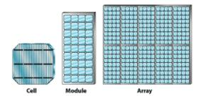
Figure 1: Solar PV Cell, Module, and Array
