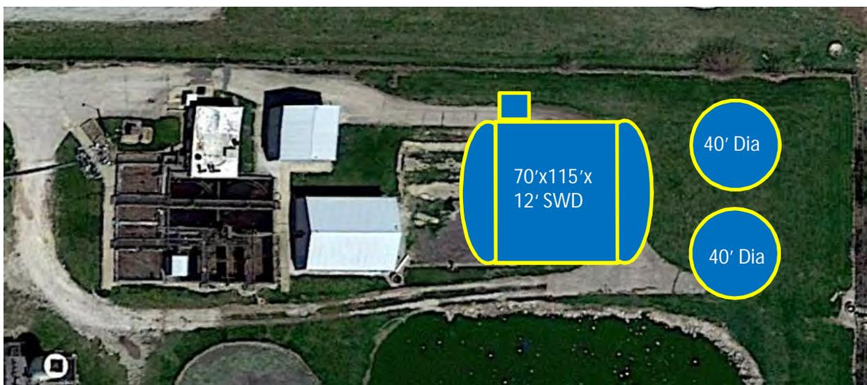
Figure 4-2 Oxidation ditch Aerial Layout
