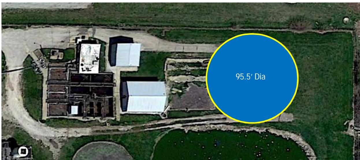
Figure 4-8 Package Plant Aerial Layout
